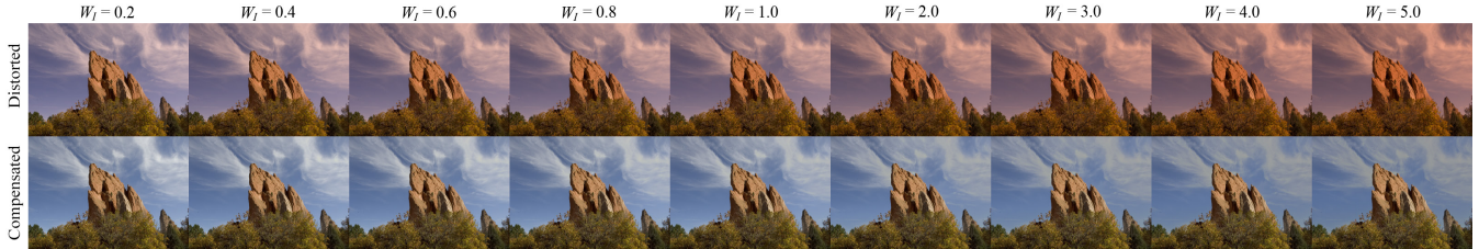
Figure 19: The distorted images in the top row demonstrate the color distortion caused by blue light blockers with different stopband widths, and the compensated images in the bottom row demonstrate the compensation quality of our algorithm.
