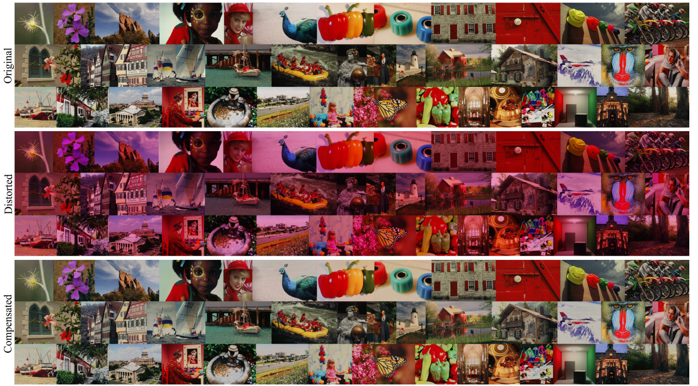
Figure 16: The original, distorted, and compensated images displayed on our prototype. All images are captured with a digital camera.
